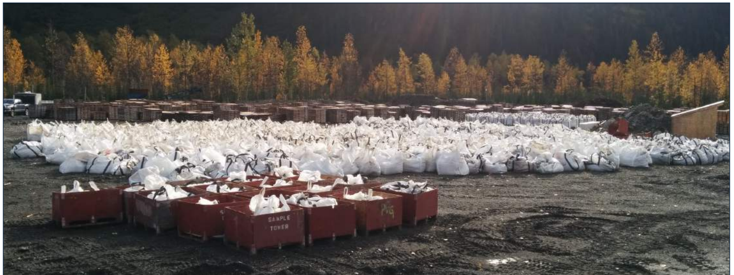
10,000 m of H cuttings recovered from the drilling fluid are bagged and ready for removal from site.
